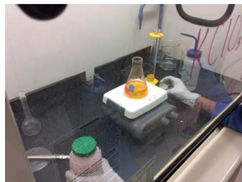
Mixing reagents under the vent hood for synthesis of chrome alum.
