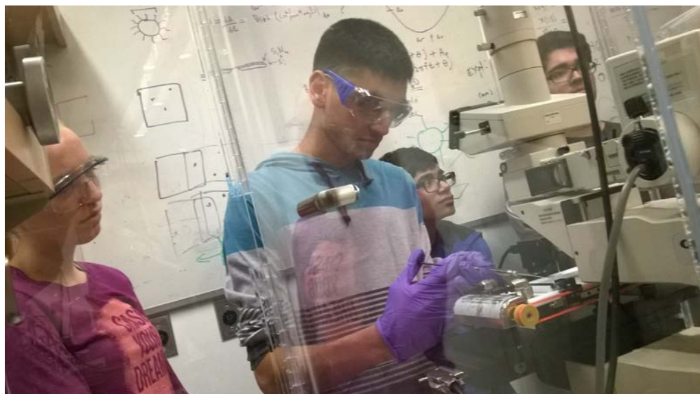
Dillon Vadgama applies the nanoparticle mixture to the liquid in the Langmuir trough.
